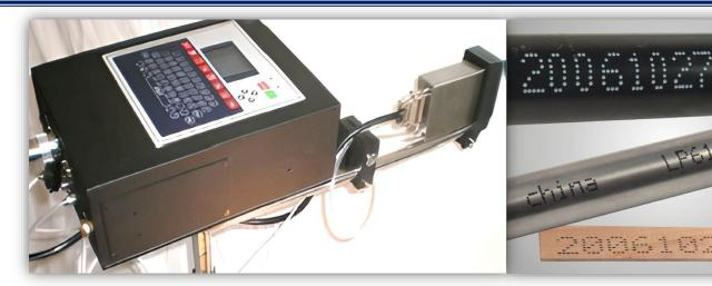
A programmable non-contact large character ink jet printer for on-line product coding & marking of both porous and non-porous products (lumber, metals, cans, plastic board, tires, etc.) in harsh environments.
