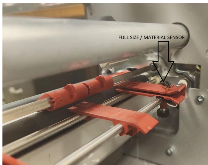
Full Size / Material Sensor before Print Head
