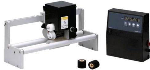
**The Series 8050-SD** is a compact rotary coder which uses instant dry thermo fusible ink rollers. It is designed to print dates, codes batch numbers, price and other variable information on all types of flexible packaging such as cellophane, polypropylene, aluminum, polyester or paperboards at speeds up to 35m/min. with a 30 x 35 mm printing area. It can be easily installed on all types of continuous motion packaging machines including flow pack units and form/fill/seal packaging machines.
