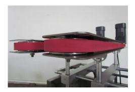
Using an Allen wrench, loosen the sprocket. This is a carriage bolt so you will not need to back the screw up with another wrench. On the inside of the rail, carefully place a flat head screwdriver between sprocket and the delrin rail, carefully prying the sprocket away from the rail, and then tighten screw. This belt does have teeth to drive it, so you do not need to over tighten it. This could shorten the life of the belt
