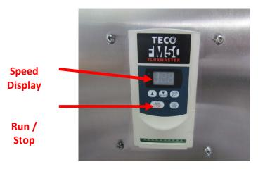
Turn your Transport Conveyor on and let it run for a little while. Now that your Transport Conveyor is set up to run your containers, the only variable is belt speed. In most circumstances you will want it to run just a little faster than the machine that feeds itwhether it's a bottle Orientator, or a filler, or capper. By running a little faster than the machine that feeds it, a gap will be created between containers, rather than having them bunch up at the entrance to this conveyor.
