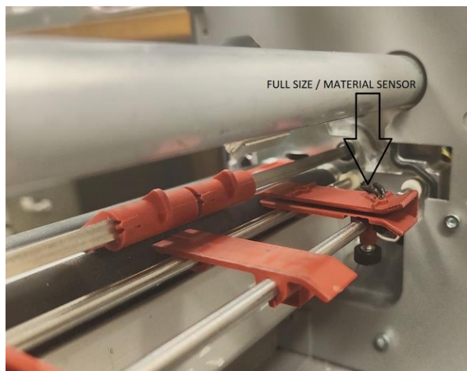
Full Size / Material Sensor before Print Head
